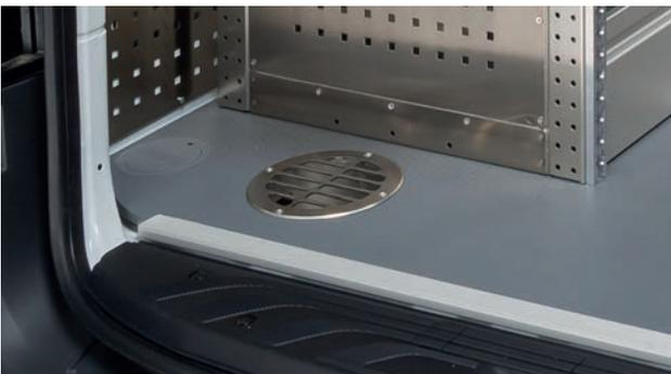
It is essential to take care when installing ventilation and venting grids on parts of the frame, electrical and/or hydraulic lines, fuel lines or fuel tanks, other floor openings etc.!
