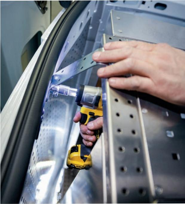
The wall fastenings must be fixed so that they are evenly loaded in tension and pressure. If the device has more than 2 supporting frames, the central fastening frame must also be fixed. Use M6 expanding rivet nuts with collar. In each case, two screws must always be fixed to the supporting frame and to the bodywork.
