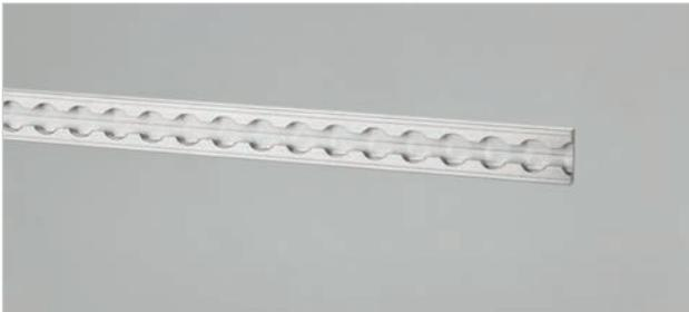
ALUCA fastens the lashing rails with M6 countersunk screws (DIN 7991) of strength 8.8 and M6 locknuts (DIN 985) or M6 expansion nuts. With a spacing of approx. 150 mm, we can guarantee pull-out force of 200 daN. We have demonstrated this by means of pull-out trials of the lashing rails in collaboration with the manufacturer.
