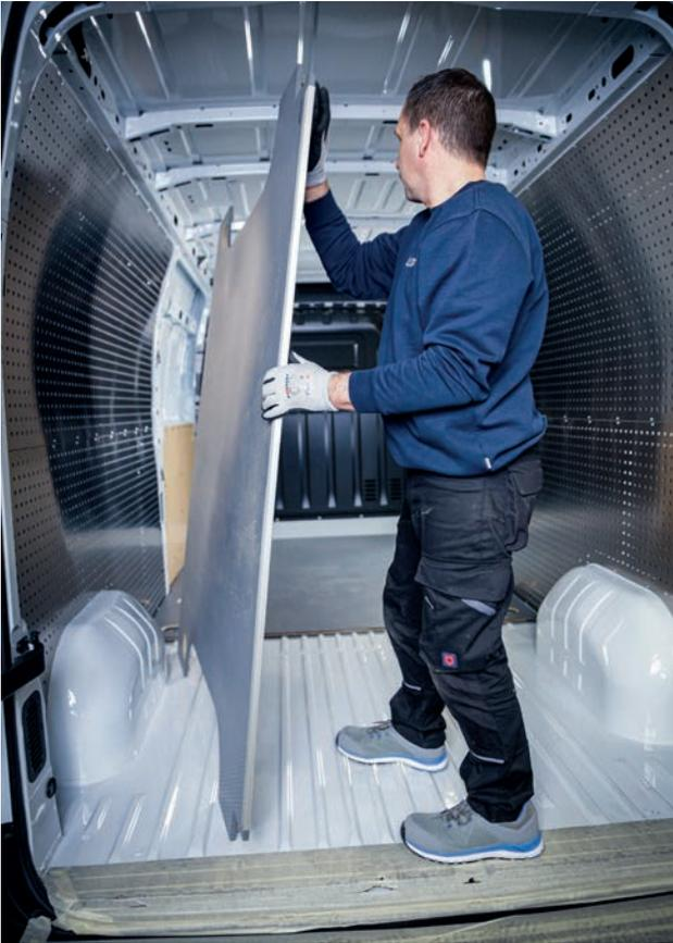
ALUCA floorplates are fixed via the original lashing points. With this, you should consider that we have developed plastic components for lashing points (pot and lid) which are used for all vehicle types.
